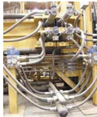
Valley Hay Co. wanted to increase the throughput of its presses, which ran at a single speed in order to compress the most difficult materials. After retrofitting controls, the presses now run at maximum speed based on the material being compressed.
